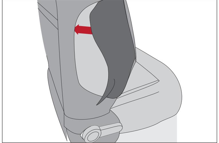
6. Press fabric down around head rest buttons until through cut outs in fabric.
