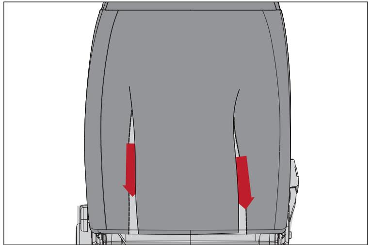
4. Push bottom fabric flap through crease in bottom of seat toward rear of vehicle and secure to rear fabric of back cover.
